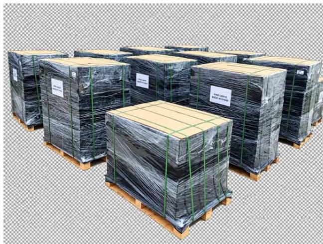
28 Wrapped and strapped shipping units on pallet bases.
